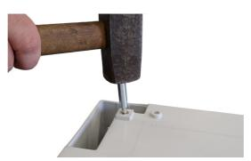
Fig. 3-3 Hammering in a drive-in nut.
