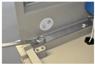
Fig. 3-11 Tighten the connecting screws (view of left side in the pedestal).
