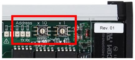
Fig. 4-3 Switches for setting the bus address.
