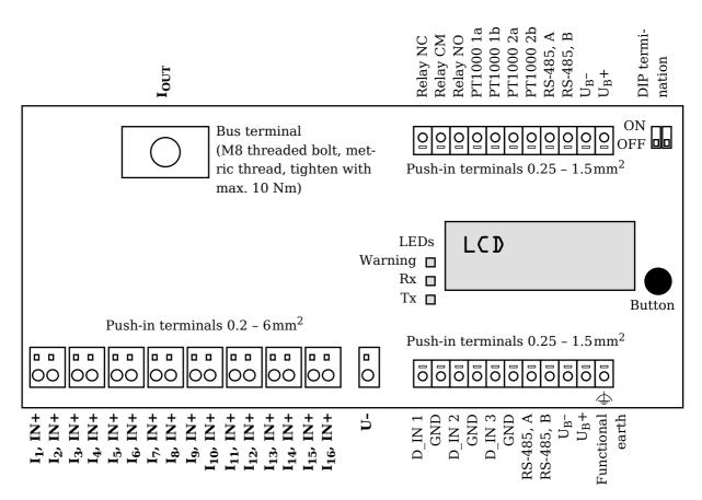
Fig. 3-2 Terminal assignment of the string.bloxx module 116 (the drawing is not drawn to scale).
