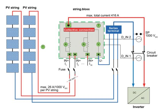
*Fig. 3-1 Typical wiring; OVP = overvoltage protection.*
