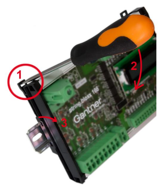
Fig. 3-3 Removing a module (example).
