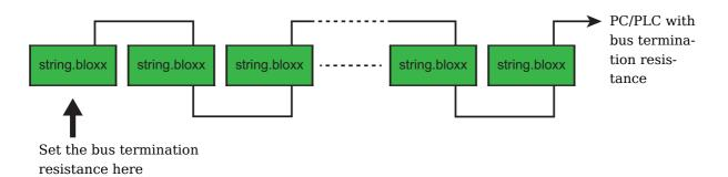
Fig. 5-1 Bus wiring for RS-485 or Modbus.
