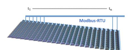
Fig. 5-3 Time offset due to serial communication in standard PV systems.
