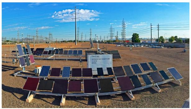
The Outdoor Test Facility (OTF) from Gantner Instruments provides all required data sets for an easy and accurate validation and technology comparison of your PV module. The OTF solution measures all parameters for energy yield, low light behavior and thermal coefficients for any PV technology in order to create track record data and bankability support.
