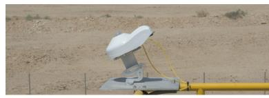
ISO 9060 Secondary Standard pyranometer No change of desiccant for 10 years Smart, more than just digital RS-485 Modbus® communication
