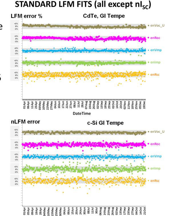
Improving **CdTe** nl<sub>sc</sub> fit from an empirical **Spectral Response** correction
